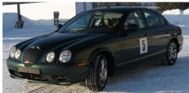
Rear-wheel drive test vehicle equipped with active front steering and differential braking used for experimental validation
