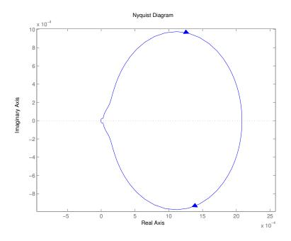
As the open-loop transfer function KP(s) is asymptotically stable, by Nyquist's criterion closed-loop stability is ensured if and only if the Nyquist diagram of KP(s) does not have clockwise encirclements of the point -1, or in other words the Nyquist diagram of P(s) does not have clockwise encirclements of the point -1/K+j0. Therefore, by restricting K to only assume positive values, closed-loop stability is always ensured.
