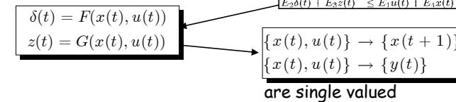
$$\begin{aligned} x(t+1) &= Ax(t) + B_1u(t) + B_2\delta(t) + B_3z(t) \\ y(t) &= Cx(t) + D_1u(t) + D_2\delta(t) + D_3z(t) \\ E_2\delta(t) + E_3z(t) &\leq E_4x(t) + E_1u(t) + E_5 \end{aligned}$$
