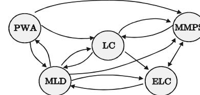
**Theorem 1** All the above five classes of discrete-time hybrid models are equivalent (possibly under additional assumptions, like boundedness of input and state variables)
