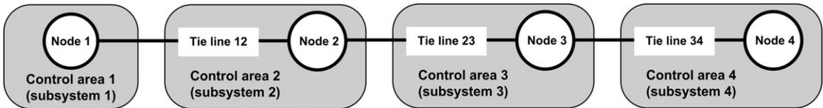
Figure 2. Schematic representation of a power network consisting of four control areas.
