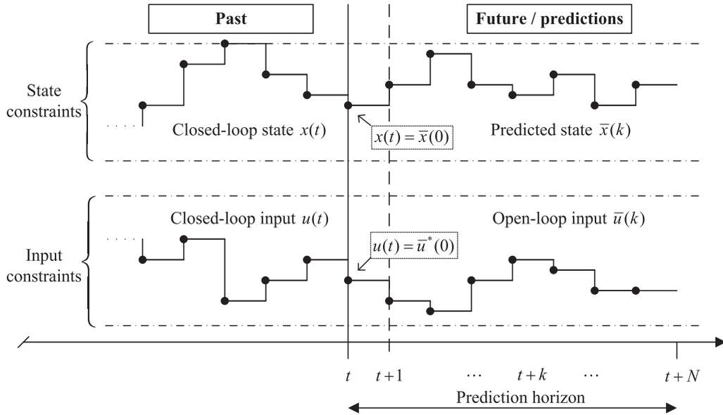
Figure 1. A schematic illustration of model predictive control.
