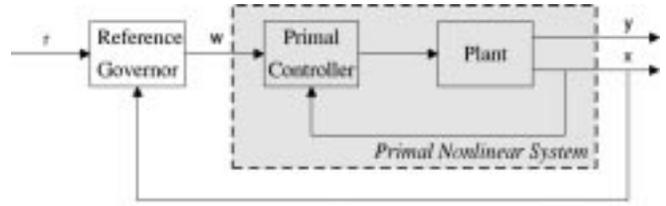
Fig. 1. Control scheme with RG.
