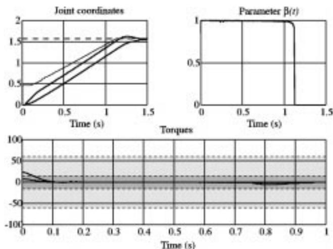
Fig. 6. Response with RG, torque constraints, and the constraint  $|\theta_1 - \theta_2| \leq 0.2$  rad. The generated reference input is depicted (thin line) together with the joint trajectories (thick lines).
