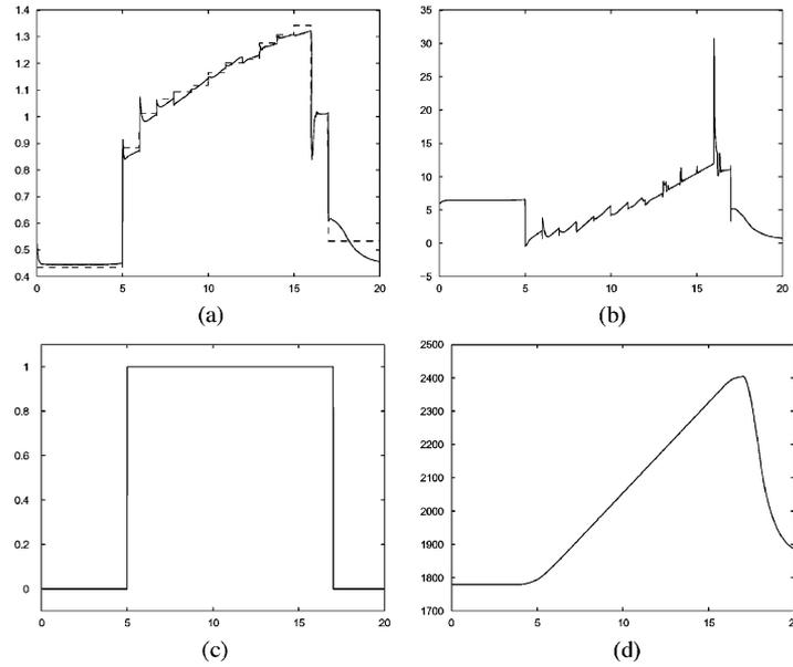
Fig. 4. Closed-loop response (nonlinear model + MPC controller) at variable engine speed. (a) Mass flow rate of fuel  $W_f(t)$  (dashed line: desired value, solid line: response of the controller). (b) Spark retard from MBT,  $\delta_{MBT}(t) - \delta(t)$ . (c) Mode of combustion  $\rho(t)$ . (d) Engine speed  $\omega$ .
