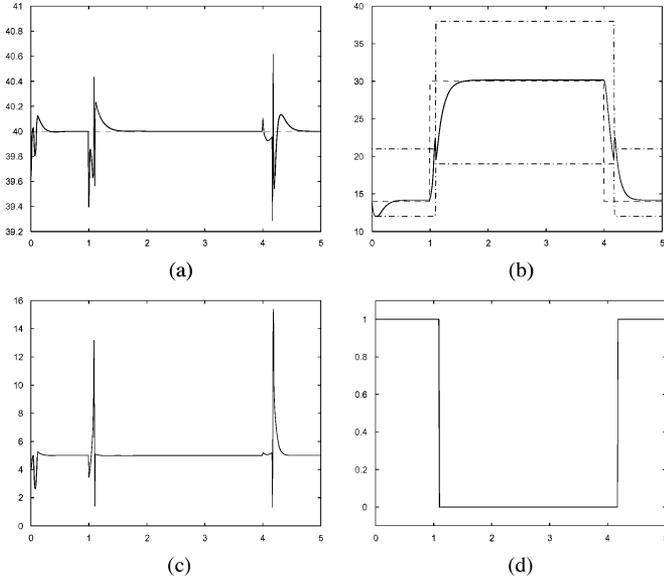
Fig. 2. Closed-loop response (nonlinear model + MPC controller) at nominal engine speed. (a) Engine torque  $\tau(t)$  (*dashed line*: desired value, *solid line*: response of the nonlinear model). (b) Air-to-fuel ratio  $\lambda(t)$  (*dashed line*: desired value, *solid line*: response of the nonlinear model, *dash-dot line*: A/F bounds). (c) Spark retard from MBT,  $\delta_{\text{mbt}}(t) - \delta(t)$ . (d) Mode of combustion  $\rho(t)$ .
