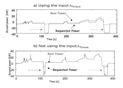
Fig. 8. Comparison between the track traction power with or without using the control signal  $\Delta_{torque}$ . Dashed arrows show the points, during both simulations, where it was impossible for the engine to reach the desiderate ground power.
