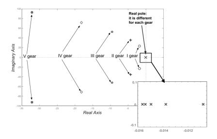
Fig. 3. Position of the poles for each gear
