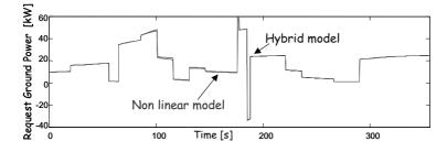
**Fig. 5.** Comparison of requested ground power: nonlinear model (1) vs. hybrid MLD model (2)
