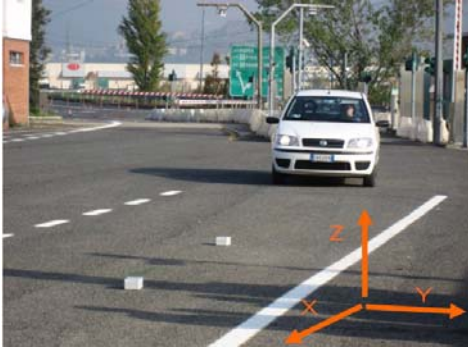
Fig. 1. Two wireless sensor nodes deployed on the road
