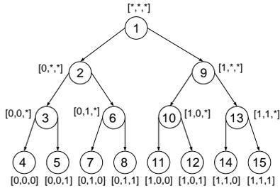
Figure 1: The binary tree for a MIQP with 3 integer variables. Each node is marked with the corresponding vector  $\xi_j$ . The numbers denote the order how the problems are solved in the depth first strategy.
