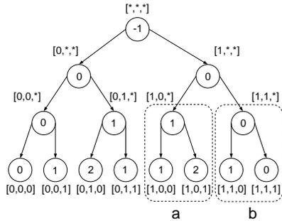
Figure 3: Number of switches for each subproblem in the outside first tree. Note the symmetry in the number of guaranteed switches of subtrees at the same depth.
