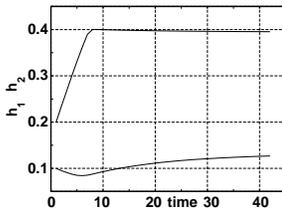
Figure 5: Trajectories of the states of the two tank system controlled by the MPC controller described by Bemporad and Morari (1999)
