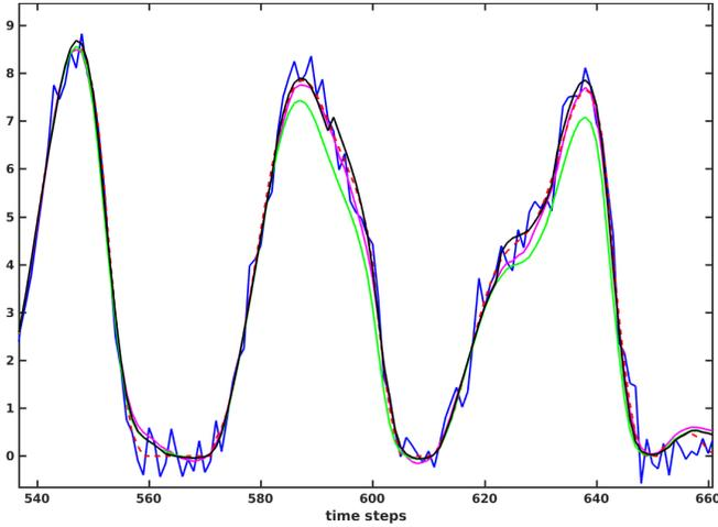
Fig. 2. Estimated output signal  $\hat{y}_k$  with  $n_x = 6$ ,  $n_a = n_b = 12$ : noise-corrupted measured signal (blue), noise-free signal (dashed red), 10-steps ahead w/ reset prediction (black), open-loop simulation (green), EKF filtered output  $y_{t|t}$  (magenta).
