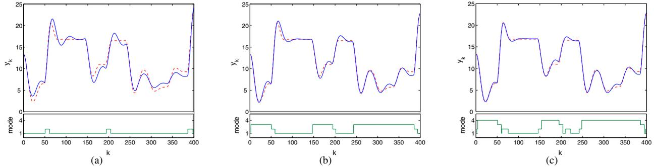
Fig. 3. Simulation results of the identified PWARX models with (a)  $s=2$ , (b)  $s=3$ , and (c)  $s=4$  submodels (solid line - simulated output, dashed line - system output). The plot at the bottom of each figure shows the evolution of the discrete mode.
