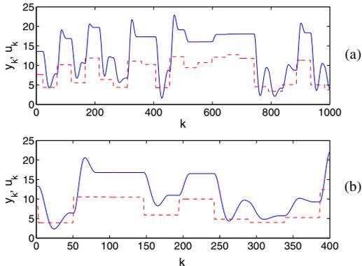
Fig. 2. Data sets used for (a) identification and (b) validation (solid line - system output, dashed line - scaled input).
