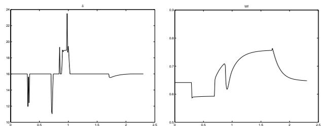
(a) Spark timing (b) Mass flow of fuel
