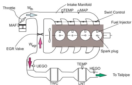
**Figure 1:** Direct Injection Stratified Charge (DISC) Engine.
