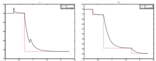
(a) Air-to-Fuel Ratio (dashed line: desired value, solid line: response of the MLD model) (b) Intake Manifold Pressure (dashed line: desired value, solid line: response of the MLD model)
