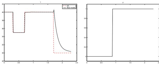
(a) Engine brake torque (dashed line: desired value, solid line: response of the MLD model) (b) Regime of combustion
