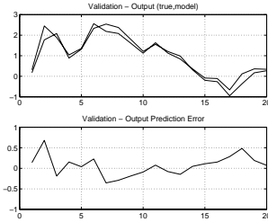
Figure 5: Identification of a linear ARX model – same estimation and validation data as in Fig. 4
