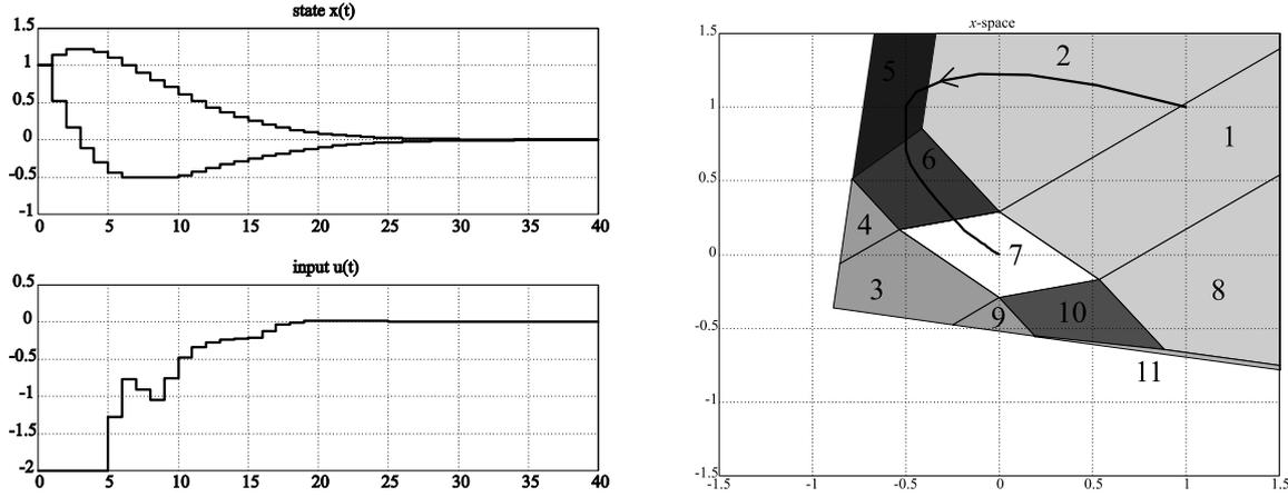
Fig. 5. Example with the additional constraint  $x_{t+k|t} \geq -0.5$ . (a) Closed loop MPC. (b) Polyhedral partition of the state-space and closed-loop MPC trajectories.
