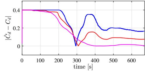
**Fig. 10.** Example 3: absolute estimation error  $|\hat{C}_d - C_d|$ . Blue:  $N = 1$ , red:  $N = 2$ , magenta:  $N = 20$ . (For interpretation of the references to color in this figure legend, the reader is referred to the web version of this article.)
