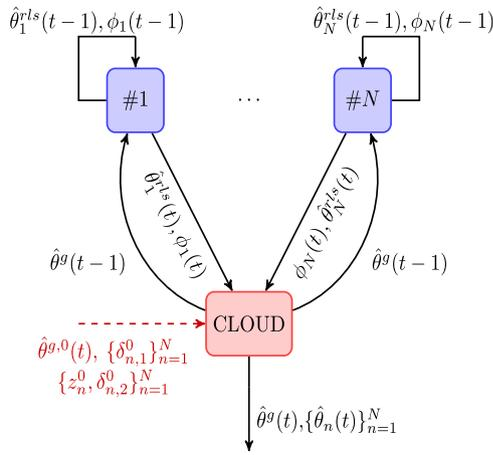
Fig. 2. Node-to-Cloud-to-Node transmissions at time  $t$ .
