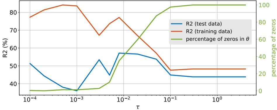
Figure 3: Average  $R^2$ -score of open-loop predictions on training/test data and model sparsity, as a function of  $\tau$ . For each value of  $\tau$ , we show the best  $\overline{R^2}$ -score obtained on test data out of 30 runs and the corresponding  $\overline{R^2}$ -score on training data and model sparsity.
