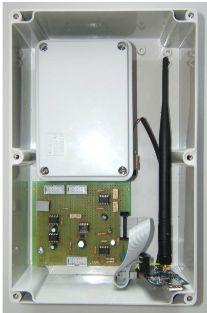
Fig. 2. Internal view of the sensor box, with electronic board and battery pack
