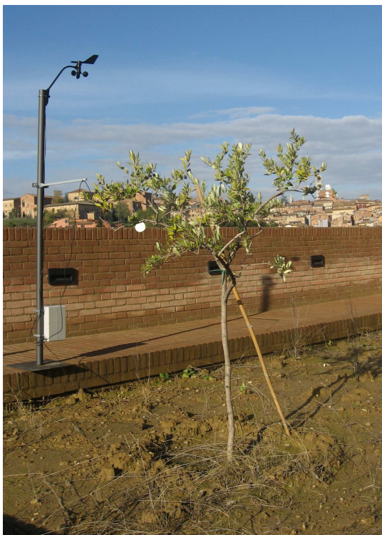
Fig. 1. Wireless acquisition station monitoring different ambient parameters of a young olive tree
