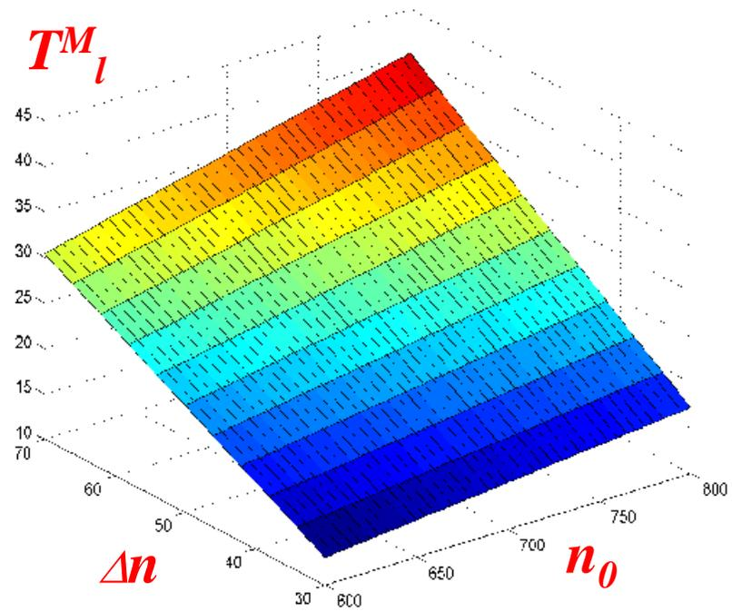
◆ **minimum** nominal engine speed  $n_0$  for which the safe set is not empty, given a range  $\Delta n$  and an upper bound on load torque  $T_l^M$ .
