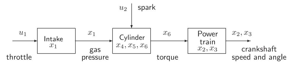
Figure. Engineering model of car engine.
